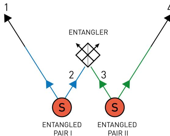
**Figure 7.** Schematic setup for an entanglement swapping experiment [22]. The two sources of entangled pairs of photons were in this case by parametric down-conversion in nonlinear crystal, which is a much more efficient source of entangled photons than can be obtained from an atomic cascade. The entangler is in the text called C for Cecilia.
