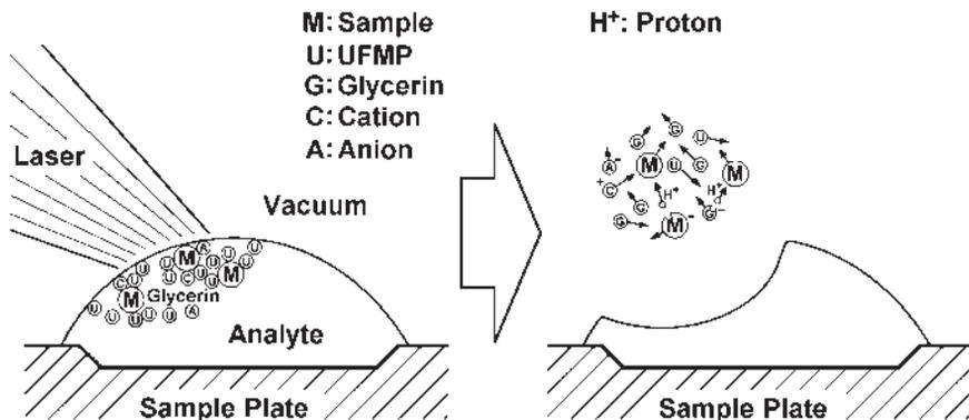
Figure 20. Macromolecule Desorption/Ionization using UFMP Glycerin Mixed Matrix.
