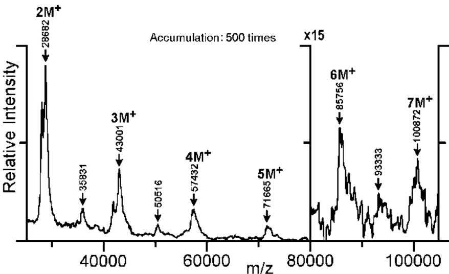
Figure 18. Cluster Ion Measurement of Lysozyme (M.W.: 14,306 Da).
