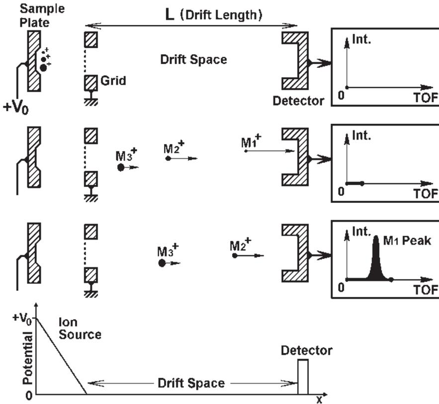
Figure 1. Schematic of Time of Flight Mass Spectrometry.
