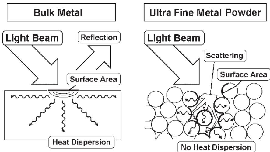
Figure 13. Differences between Bulk Metal and Ultra Fine Metal Powder.
