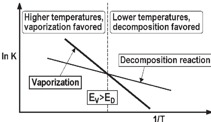
Figure 12. Vaporization vs. Decomposition.<sup>[9]</sup>
