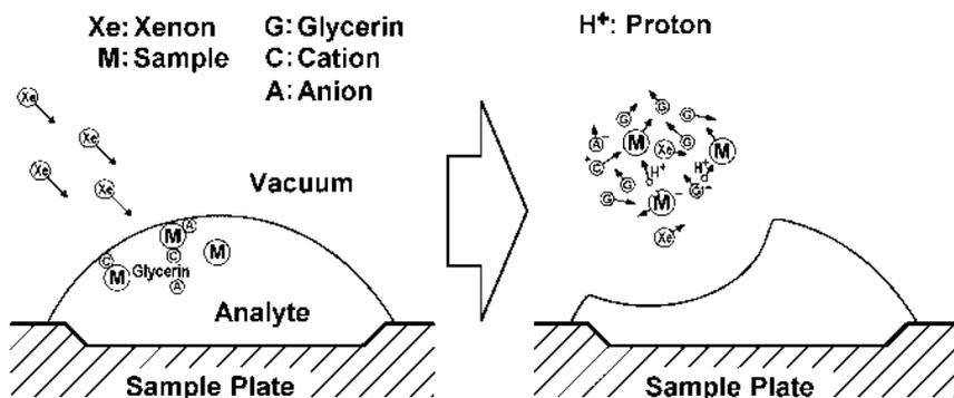
Figure 16. Molecule Desorption/Ionization using Glycerin Matrix in FABMS.
