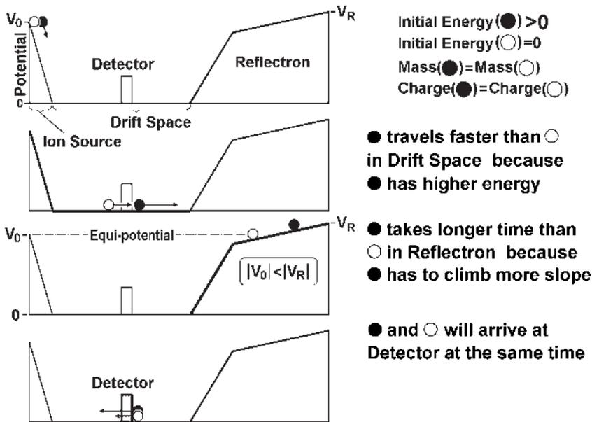
Figure 2. Mass Resolution Improvement by Reflectron.
