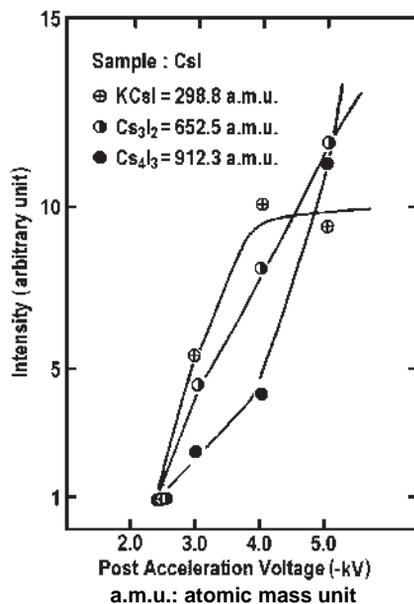
Figure 7. High Sensitivity Ion Detection by Post Acceleration.
