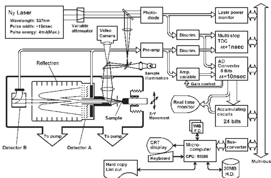
Figure 10. Schematic of Shimadzu LDI-TOFMS.
