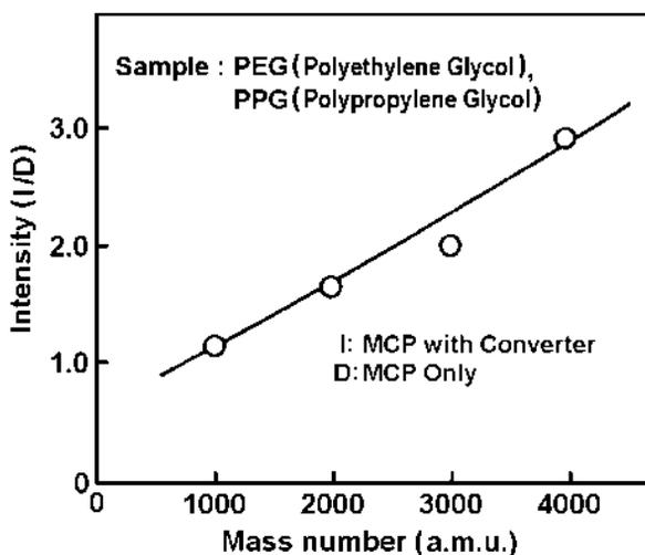
Figure 8. High Sensitivity Ion Detection by Ion-to-Electron Conversion.
