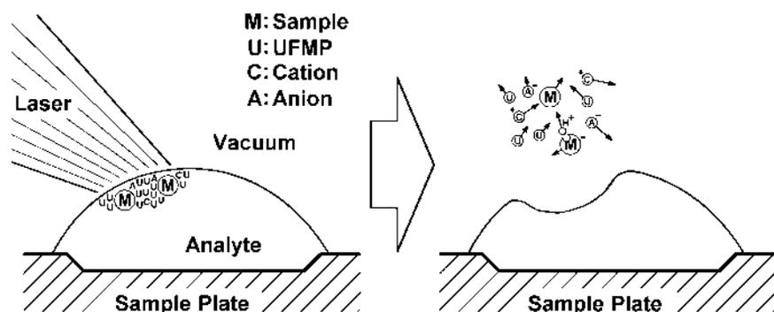
Figure 14. Molecular Ion Desorption by using UFMP Matrix.
