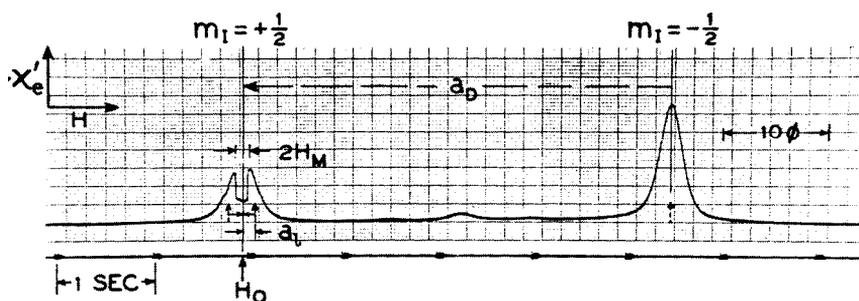
DEMONSTRATION OF THE INHOMOGENEOUS BROADENING IN P-DOPED SILICON ( $\rho = 0.25 \Omega \text{ CM}$ ,  $T = 1.2^\circ \text{ K}$ ,  $H_0 = 3000 \phi$ ) IN THE ENDOR TECHNIQUE SPIN PACKETS ARE FLIPPED AS INDICATED BY ARROWS
