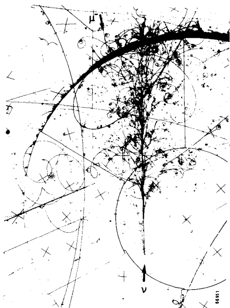
Figure 3 A typical neutrino event as observed in the Big European Bubble Chamber (BEBC) filled with neon at the CERN 450 GeV Super Proton Synchrotron (SPS) accelerator. The muon can be seen on the left. It has been tagged by an external muon identifier. The many-particle hadron shower is to the right.
