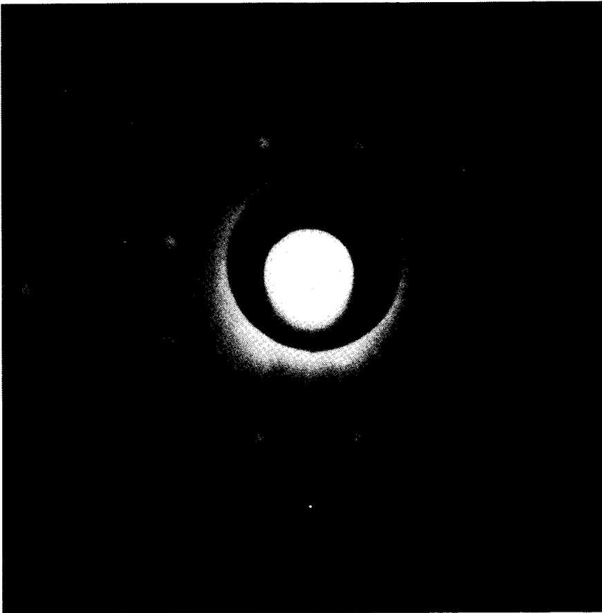
Fig. 9: Neutron Laue Pattern Taken with NaCl Crystal
