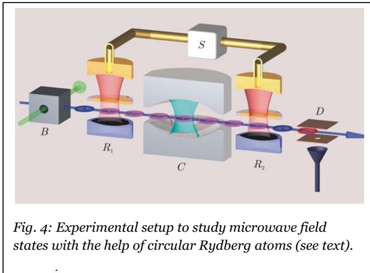
Fig. 4: Experimental setup to study microwave field states with the help of circular Rydberg atoms (see text).
