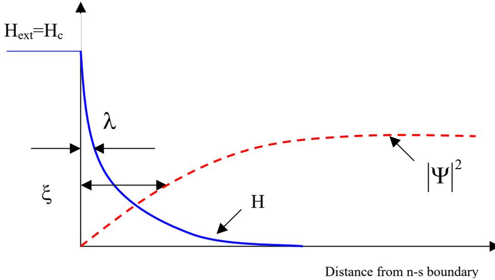
**Figure 3.** Sketch of the border region between a normal and a superconducting phase, illustrating the concepts of penetration length  $\lambda$  and coherence length  $\xi$ . If the magnetic field is  $H_c$  in the normal phase, it decays to zero in the superconducting phase over a length  $\lambda$ . At the same time the superconducting order increases from zero at the interface to its full value inside the superconducting phase over a distance  $\xi$ .
