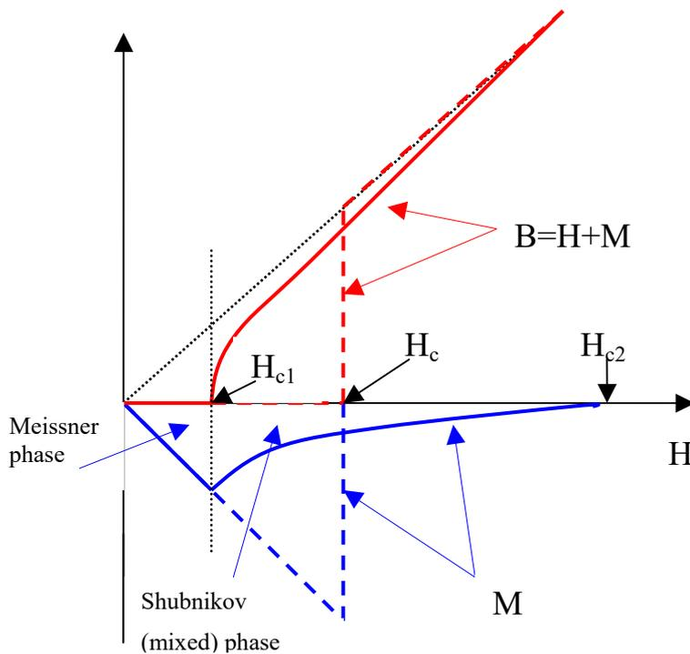
**Figure 2.** (Colour) Magnetisation  $M$  (blue) and induced field  $B$  (red) as a function of external magnetic field  $H$  for superconductors with complete (dashed lines) and partial (full lines) Meissner effect (see text).
