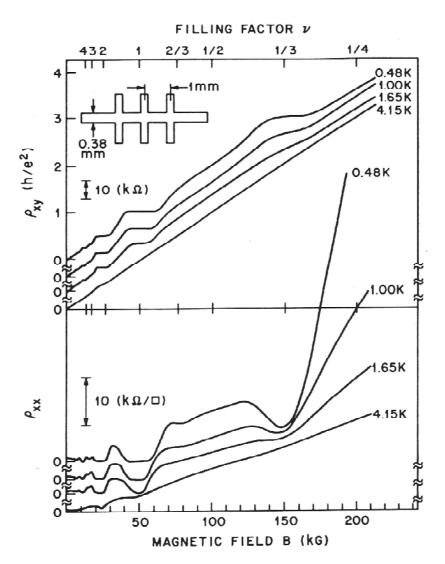
Graph showing the results of the original experiment where the fractional quantum Hall effect was discovered for filling factor f=1/3, around which the Hall resistance has a plateau at low temperatures. In later experiments well defined plateaus appeared also at many other filling factors, accompanied by much sharper minima in the Ohmic resistance than shown for the 1/3 case in the lower panel here (see figure in the press release at http://www.nobel.se/announcement-98/physics98.html).
