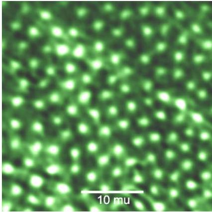
**Figure 4.** Abrikosov lattice of magnetic flux lines (vortices) in NbSe<sub>2</sub> – a type-II superconductor - visualised by magneto-optical imaging. The first pictures of such a vortex lattice were taken in 1967 by U. Essmann and H. Träuble, who sprinkled their sample surfaces with a ferromagnetic powder that arranges itself in a pattern reflecting the magnetic flux line structure.
