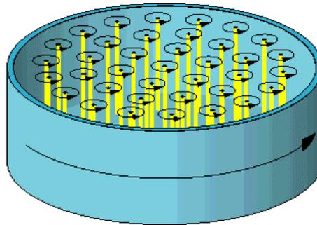
**Figure 5.** Vortex lines in a superfluid are analogous to the flux lines that occur in a type-II superconductor when it is placed in a magnetic field (Cf. Fig. 4). The picture illustrates vortex lines in rotating superfluid  $^3\text{He}$ , where the vortex structure is particularly rich. The vortex lines are shown in yellow, and the circulating flow around them is indicated by arrows.
