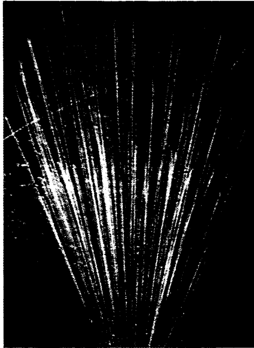
Fig. 5. Transmutation of nitrogen. The range of the alpha particle before the collision is only 3.4 cm and the range of the ejected proton, moving to the left and slightly backward, is only about 3.5 cm. The end of the 4.8 cm alpha particles from Thorium B + C can be seen near the middle of the photograph. (Blackett and Lees, 1932)
