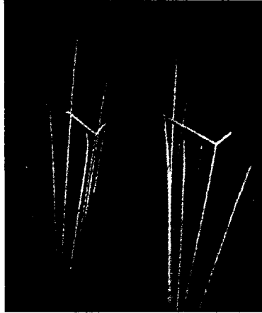
Fig. 1. Elastic collision of alpha particle with an oxygen nucleus.
