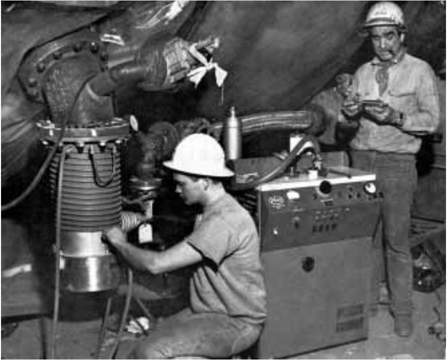
Figure 6. The entire tank was vacuum leak-tested by Chicago Bridge and Iron engineers. A small mass spectrometer capable of sensitive detection was connected to the vacuum pump and helium was introduced around the tank and all the plumbing. From Sharp Bits , September 1966.
