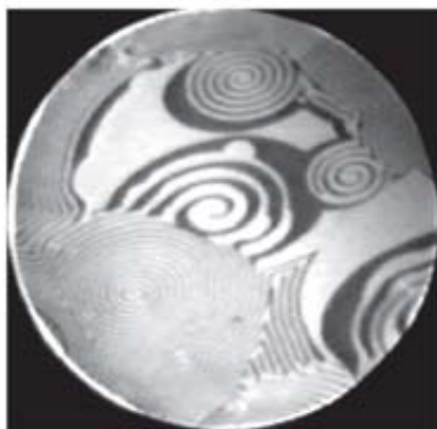
PEEM images with 500 \mu\text{m} diameter, steady-state conditions: p_{\text{O}_2} = 4 \times 10^{-4} mbar, p_{\text{CO}} = 4.3 \times 10^{-5} mbar, T = 448 K
