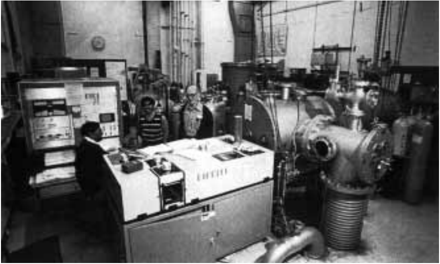
Figure 1. The “big” molecular beam system, with two “32” diffusions pumps and one “16” Jet Booster Pump, after it was moved from Princeton to Yale. The people, from left to right: S.P. Venkateshan and S. B. Ryali, both postdocs from India.
