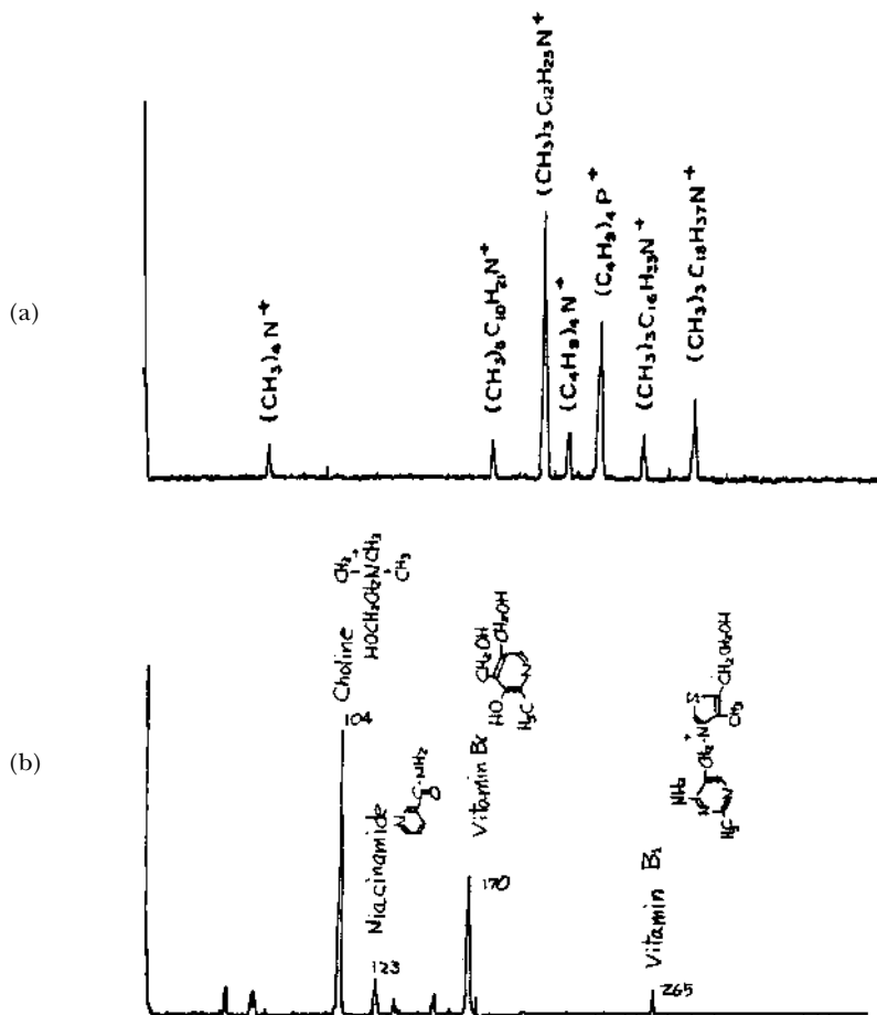
Figure 9. (a) The mass spectrum obtained with the apparatus of Figure 8 with a dilute solution (ppm) of quaternary ammonium halides and one quaternary phosphonium halide in 50-50 methanol water. (b) The mass spectrum obtained with a solution obtained by dissolving a vitamin B tablet in 50-50 methanol water.
