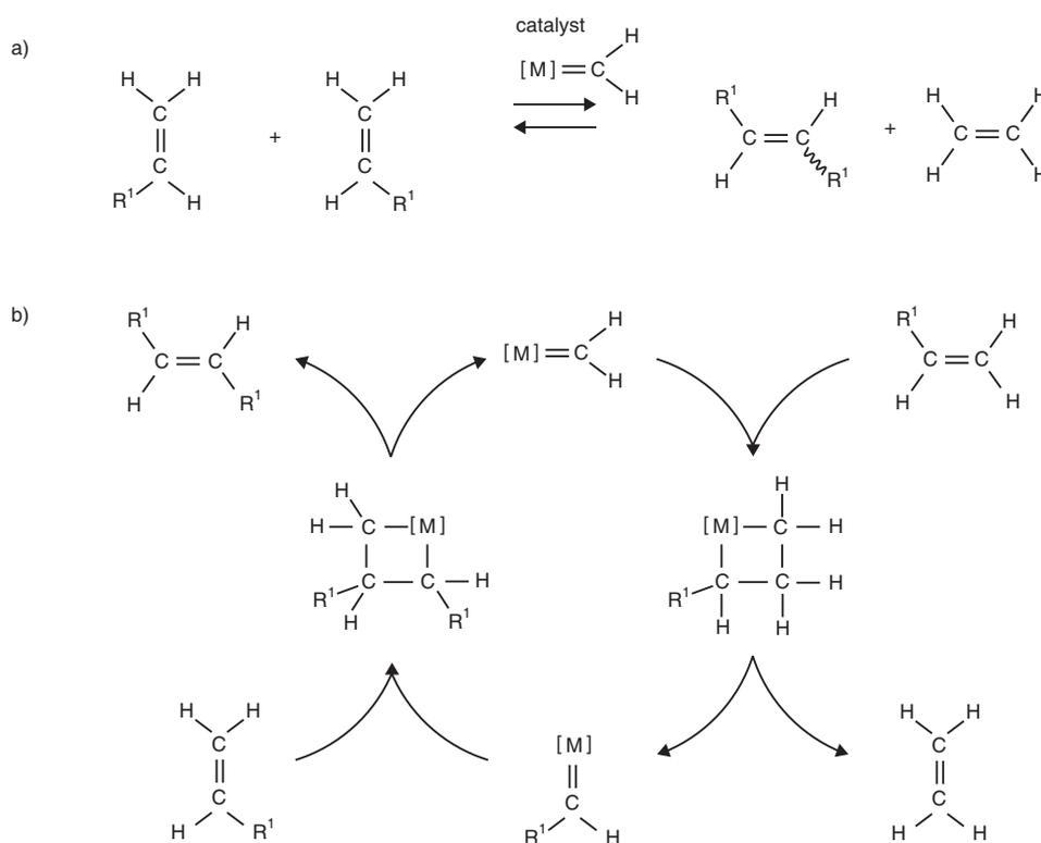
Figure 3. (a) Metathesis of alkenes catalysed by a metal alkylide. The products are two new alkenes – ethene and the alkene with two R<sup>1</sup> groups – one on each carbon in the double bond. The wavy bond shows that the R<sup>1</sup> groups can be located on the same side of the double bond or on different sides. (b) Chauvin's mechanism for olefin metathesis. In the catalytic cycle on the way to the products rings with four atoms are formed – three carbons and one metal.
