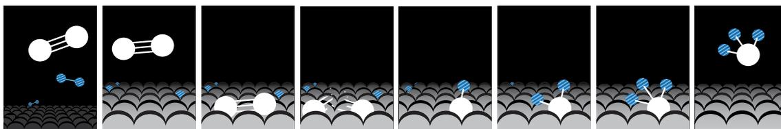
*In the Haber-Bosch process nitrogen (white) reacts with hydrogen (striped) on an iron surface to then form molecules of ammonia which are released from the surface. This reaction, which extracts nitrogen from air, is an important step in the production of artificial fertilizer.*
