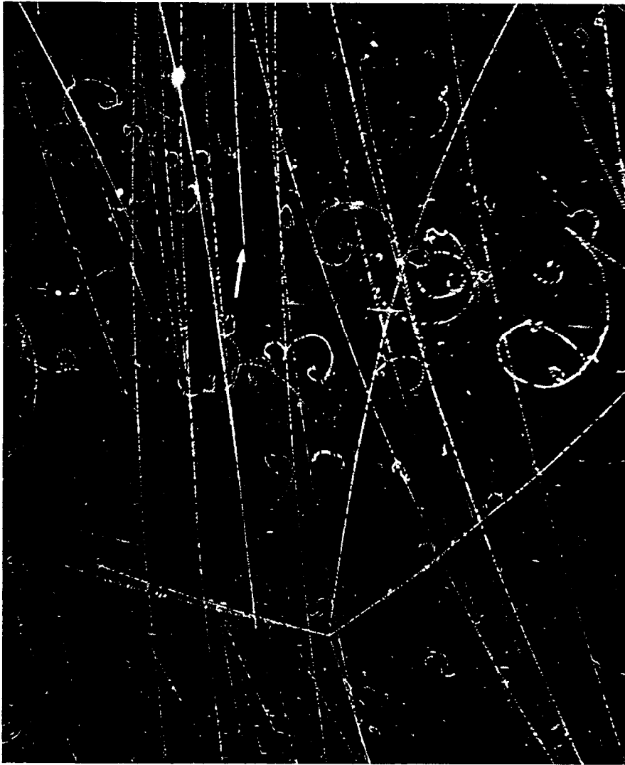
Fig. 1. An antiproton enters a propane bubble chamber, and at the point marked with an arrow undergoes charge exchange. The antineutron originates the annihilation star (directly below). Density of propane 0.42 \text{ g/cm}^3 . Real distance between charge exchange and origin of star 9.5 \text{ cm} . T_{\bar{p}} at charge exchange \sim 50 \text{ MeV} . (From Agnew et al. 5 )
