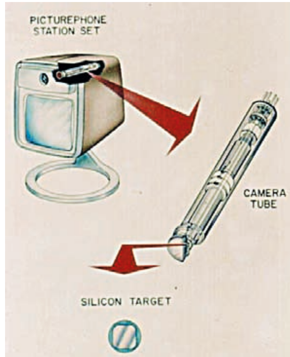
Figure 2. The Picturephone set and silicon diode array camera tube.
