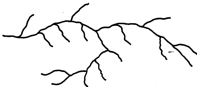
Fig. 4. High-pressure polyethylene, structural principle.
