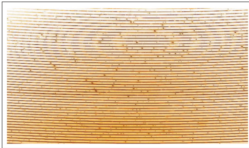
Figure 2. Middle cut of ELODIE image of a stellar spectra observed with simultaneous thorium recorded on the CCD. One clearly distinguishes the curved spectroscopic order of the stellar spectra from the interlaced emission spectrum due to simultaneous thorium lamp illuminating the second fiber.
