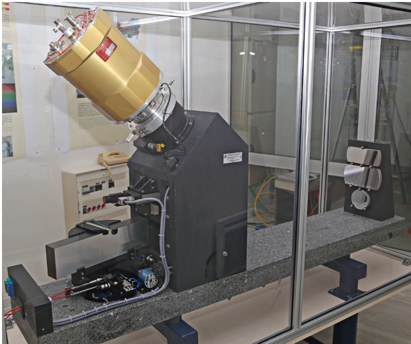
Figure 1. ELODIE spectrograph on display at OHP. On the left we see the échelle grating with the grooves facing us. On the left side, the optical fibers feeding the spectrograph are clearly visible (in orange). On the top sits the cryostat with the CCD detector inside. The “cross-dispersing” optic (not visible) is located in the vertical dark painted holding structure. ©Collection Photothèque OHP/CNRS.
