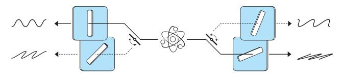
**Alain Aspect** developed this experiment, using a new way of exciting the atoms so they emitted entangled photons at a higher rate. He could also switch between different settings, so the system would not contain any advance information that could affect the results.
