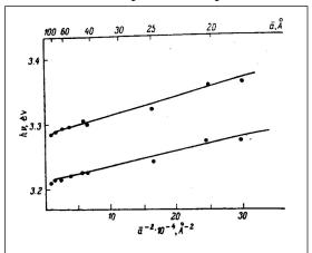
Fig. 2. Dependence of the spectral positions of exciton absorption lines at T = 4.2 K on the average radius  $a^-$  of CuCl nanocrystals in glass. The energy of the absorption line increases proportional to  $^{-2}$ . Reproduced from A.I. Yekimov and A.A. Onushchenko, *JETP Lett* 1981, *34*, 345–349.
